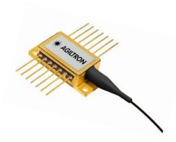
The 1440nm series laser diodes are fabricated in a hermetically sealed 14-pin butterfly package. The laser diodes contain a monitor photodiode, thermoelectric cooler (TEC), and a thermistor to secure high-quality laser performance. Our laser products are Telcordia GR-468 qualified and in compliance with RoHS Directives.
